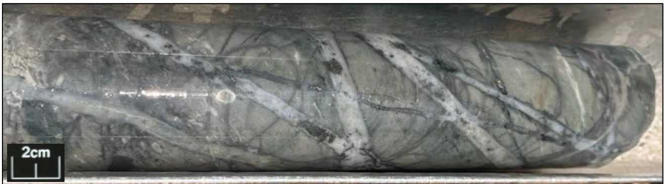
Figure 1: Stockwork quartz (~85%) – pyrite (~15%) veins at ~156 m downhole in 26DDRM006 at Rohav Mountain. Assays are pending for this hole. Visual estimates of mineral abundance should never be considered a proxy or substitute for laboratory analyses where concentrations or grades are the factor of principal economic interest. Visual estimates also potentially provide no information regarding impurities or deleterious physical properties relevant to valuations.
