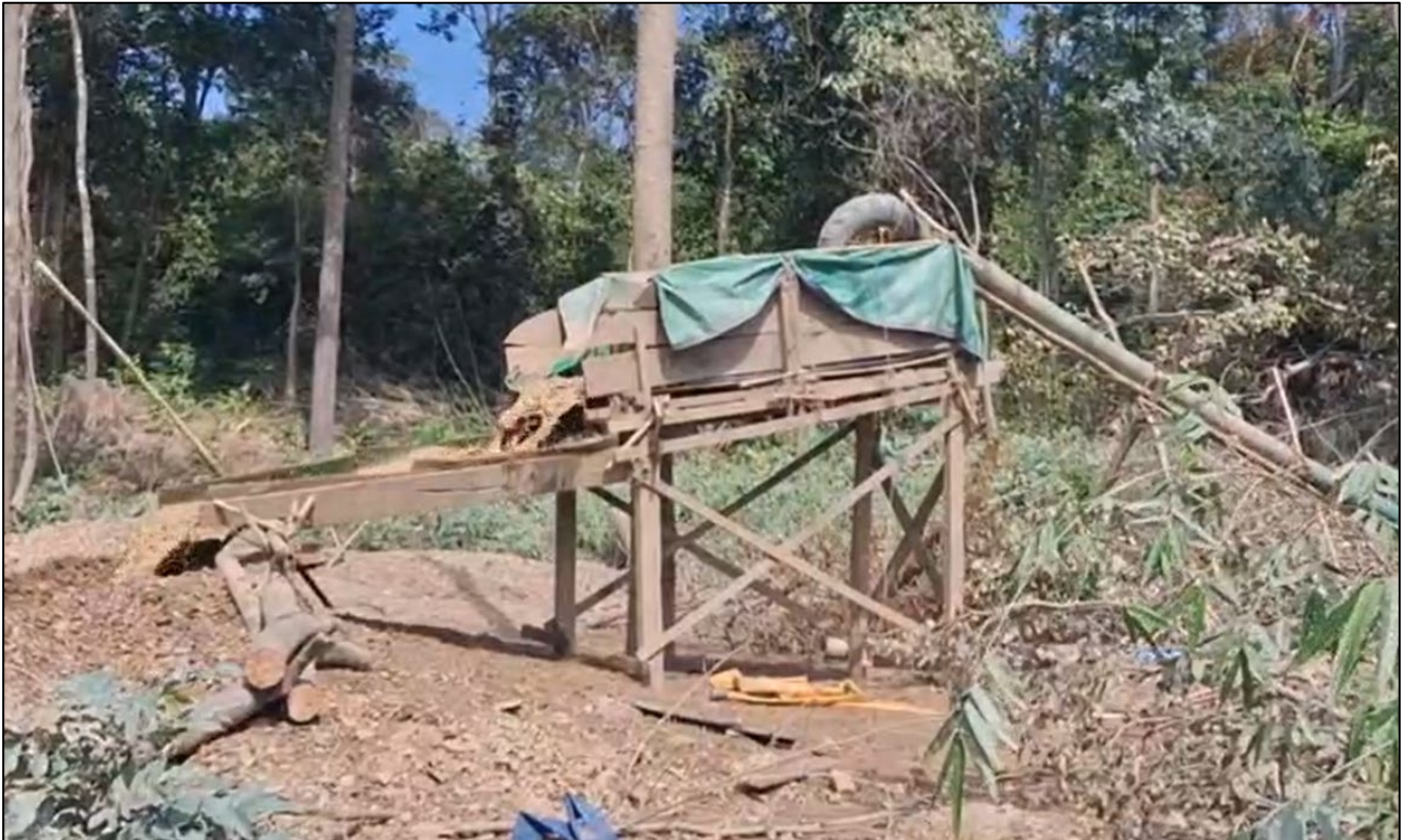
Figure 10: Artisanal wash plant treating alluvium at the Rohav Mountain Prospect.
