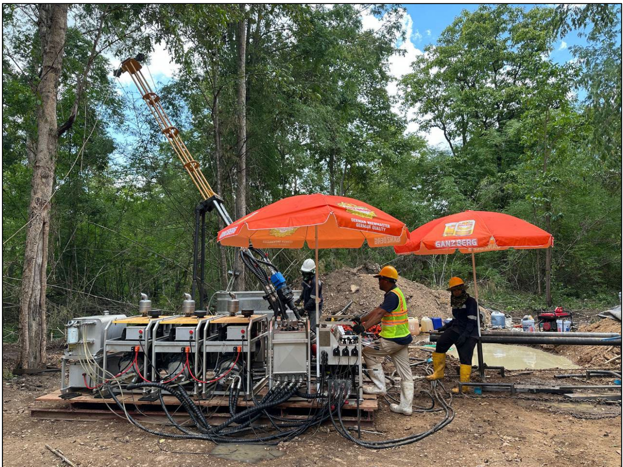
Figure 4: Unity’s first drill hole (26DDCM001) at the Camp Prospect is underway. The Company is utilising a man portable rig to enable the drilling to continue into the monsoon season as long as practicable.
