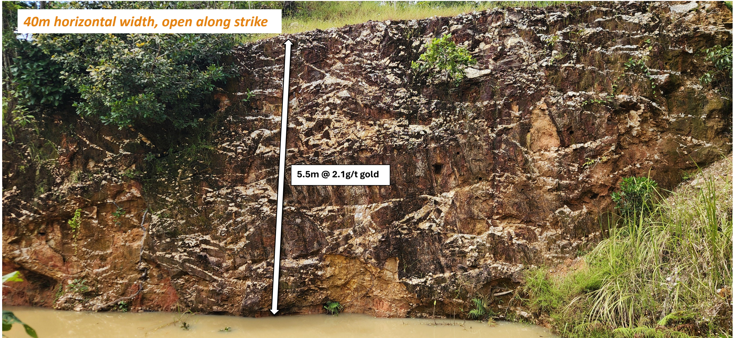
Unity channel sampling of stockwork vein mineralisation hosted in granodiorite at Camp Prospect
