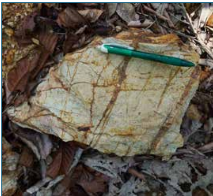
Photograph 11: (Left) Srolao Prospect. Stockwork gold-bearing quartz-arsenopyrite mineralisation in sediments from the area of the main artisanal workings. A rock chip sample (ID 103025) taken from this mineralisation at location 695045 m East, 1392882 m North returned assay results of 6.8 g/t gold, 9.4% arsenic and 118 g/t bismuth (refer to Appendix A for all rock chip sample assay results). Source: Author.
