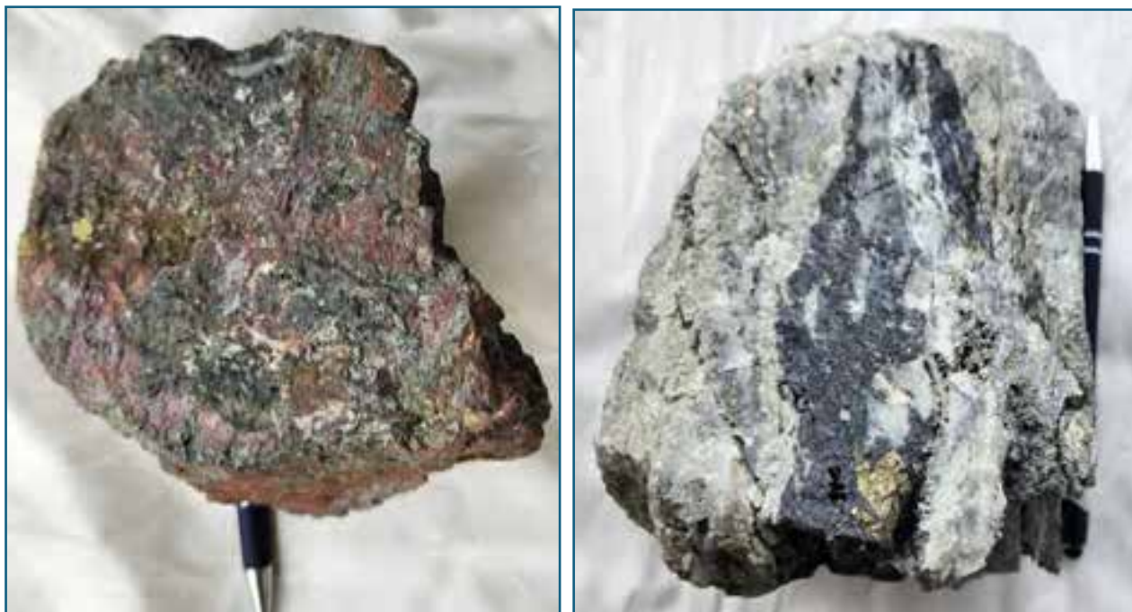
Photograph 7: (Left) Ngot Central Prospect. Float sample of diorite with chalcedonic quartz veins and quartz vein breccia with disseminated chalcopyrite and possibly cuprite. A rock chip sample (ID N2303048) taken from this mineralised diorite at location 689112 m East, 1391672 m North returned assay results of 44 g/t gold, 119 g/t silver and 1.1% copper (refer to Appendix A for all rock chip sample assay results). Source: Unity Metals.
