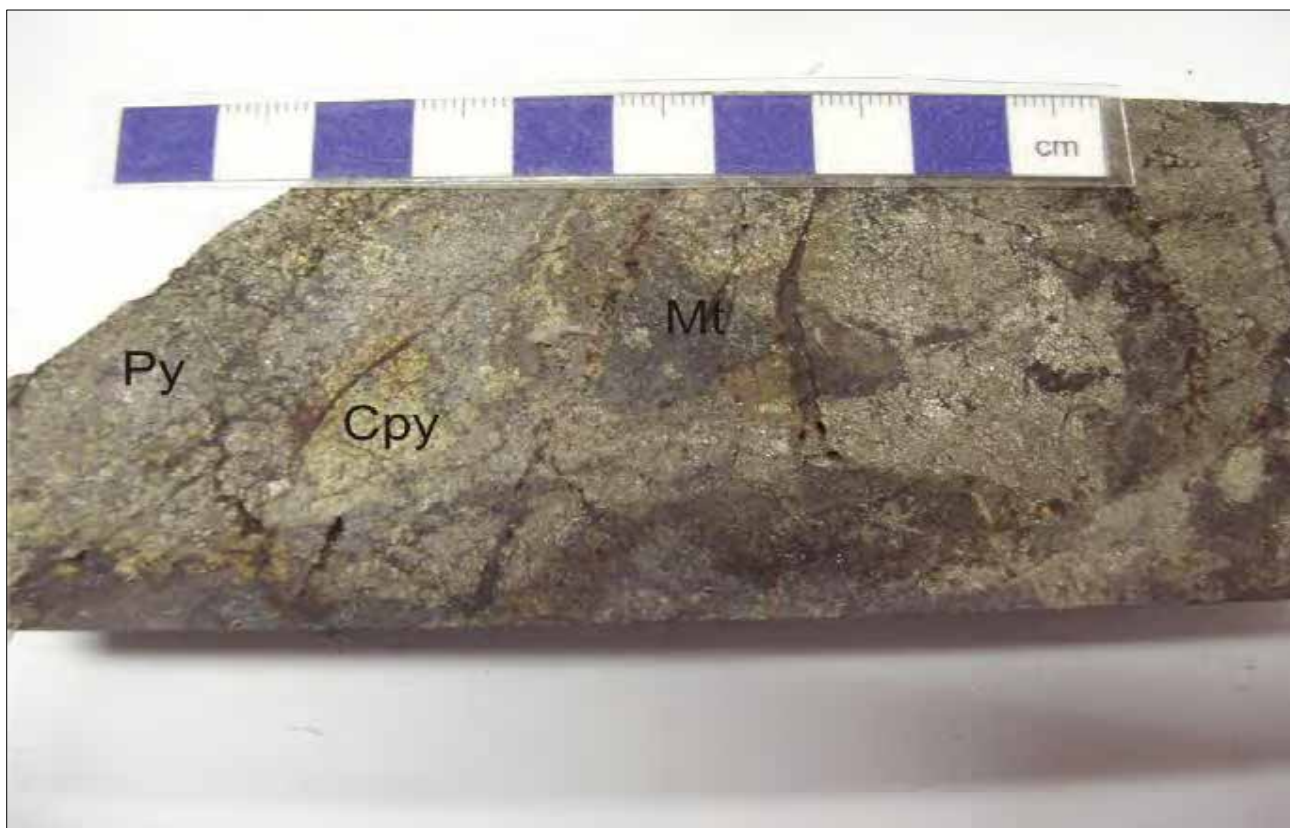
Photograph 32: PUT 2 chalcopyrite mineralisation in association with pyrite and magnetite. Source: Khositanont, 2007.
