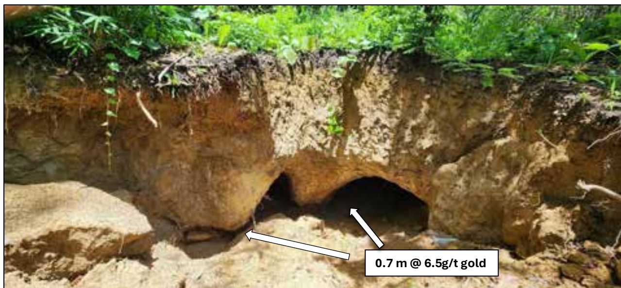
Photograph 5: Ngot Central Prospect. New artisanal workings on shallow-dipping, stacked high-grade gold veins hosted in weathered diorite (2 m below surface). The vertical composite channel rock chip result of 0.7 m @ 6.5 g/t gold was obtained from the sampling of these veins at location 689585 m East, 1391967 m North (refer to Photograph 6 for individual channel sample locations, Appendix A for all rock chip sample assay results). Source: Unity Metals.
