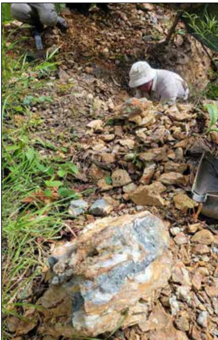
Photograph 4. Recent artisanal workings on a 40 cm wide, sheeted, quartz-arsenopyrite vein hosted in sediments at the Srolao Prospect. A grab rock chip sample taken from this vein returned 5.9 g/t gold (sample number 103031). Details on the results of Unity Metals' sampling of this vein are provided in the Independent Geologist's Report. All of the rock chip sample results from the Ngot Gold Project are provided in Appendix A of that report.
