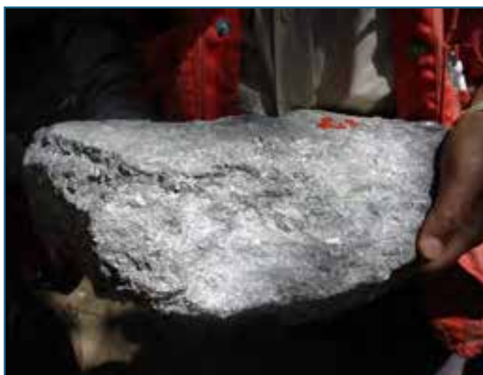
Photograph 14: (Left) 2008 Mesam Gold Mine visit. Mine dump sample of a quartz-pyrrhotite-chalcopyrite vein. Source: Author.
