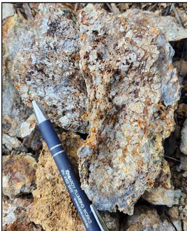
Photograph 21: (Left) Camp Prospect. Brecciated massive arsenopyrite mineralisation hosted in granodiorite from the old mine workings. A rock chip sample (ID O2303032) taken from this mineralisation at location 722747 m East, 1416171 m North returned assay results of 1.2 g/t gold, 24.4 g/t silver and 6.8% arsenic (refer to Appendix B for all rock chip sample assay results). Source: Unity Metals.
