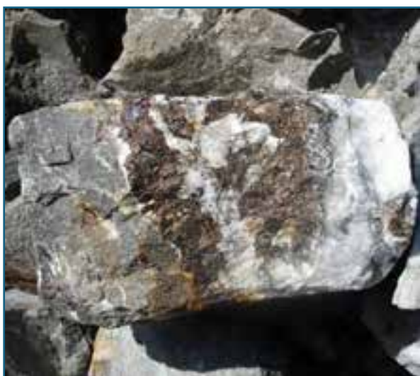
Photograph 14: (Left) 2008 Mesam Gold Mine visit. Mine dump sample of a quartz-pyrrhotite-chalcopyrite vein. Source: Author.
