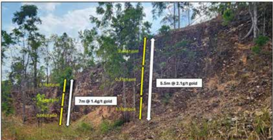
Photograph 7. Historical gold workings at the Camp Prospect on intense stockwork quartz-arsenopyrite vein mineralisation hosted in granodiorite (looking SW). Given the shallow dip of the mineralisation, Unity Metals collected vertical channel rock chip samples from exposed pit walls. Composite channel rock chip sample results include 5.5 m @ 2.1 g/t gold (sample numbers 02303021 – 02303023) and 7 m @ 1.4 g/t gold (sample numbers 02303018 – 02303020). Details on the results of Unity Metals' sampling of this mineralisation are provided in the Independent Geologist's Report. All of the rock chip sample results from the O'Phlay Gold Project are provided in Appendix B of that report.
