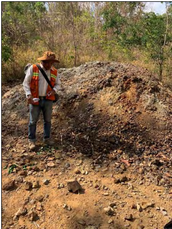
Photograph 26: (Left) Small Creek Prospect. Arsenopyrite-rich mullock adjacent to an old mine working. A rock chip sample (ID O2303062) taken from this mineralisation at location 761997 m East, 1414404 m North returned assay results of 10.7 g/t gold, 32.5 g/t silver, 26.2% arsenic and 232 g/t bismuth (Appendix B for all rock chip sample assay results). Source: Unity Metals.
