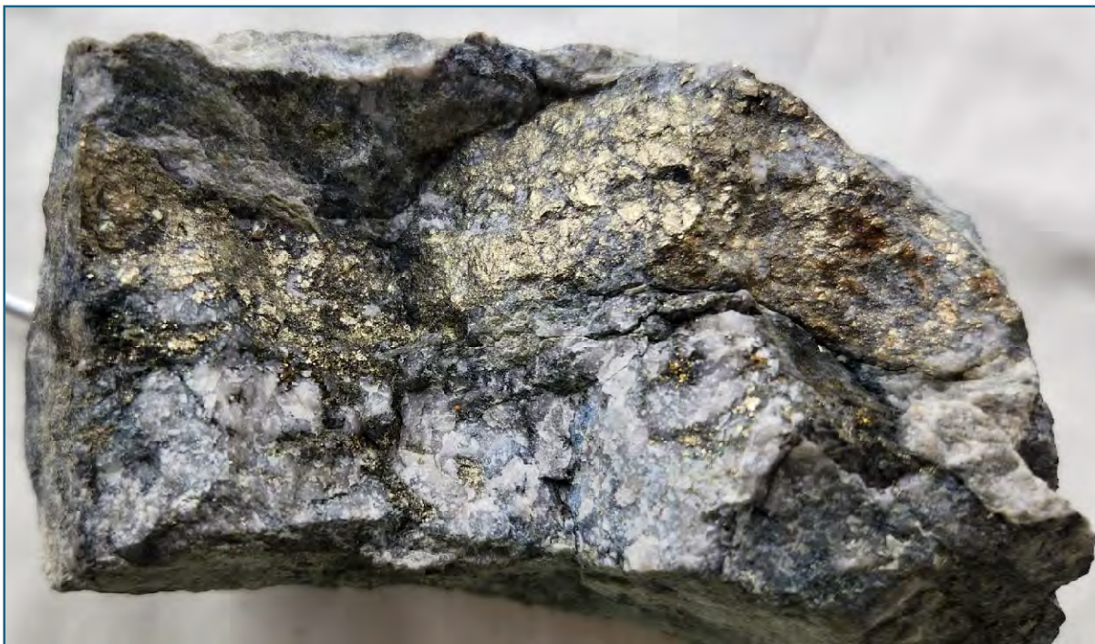
Photograph 16: Gold-bearing quartz-pyrite-pyrrhotite-chalcopyrite vein that extends south-southwest from the Mesam Gold Mine towards the Ngot Gold Project. A rock chip sample (ID N2306010) taken from this vein in artisanal mine workings at location 703318 m East, 1393559 m North (200 m outside the Ngot Gold Project) returned assay results of 6.2 g/t gold, 202 g/t silver, 1.3% copper and 680 g/t bismuth (refer to Appendix A for all rock chip sample assay results). Source: Unity Metals.
