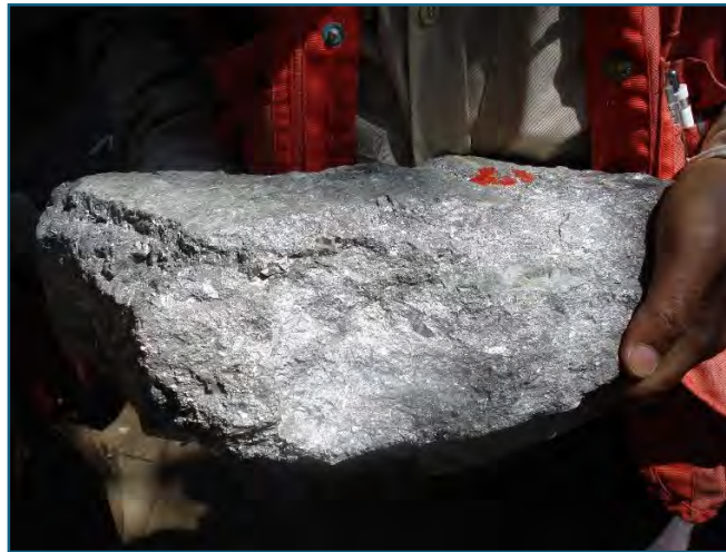
Photograph 14: (Left) 2008 Mesam Gold Mine visit. Mine dump sample of a quartz (~60%) - pyrrhotite (~40%) - chalcopyrite (trace) vein. Source: Author.
