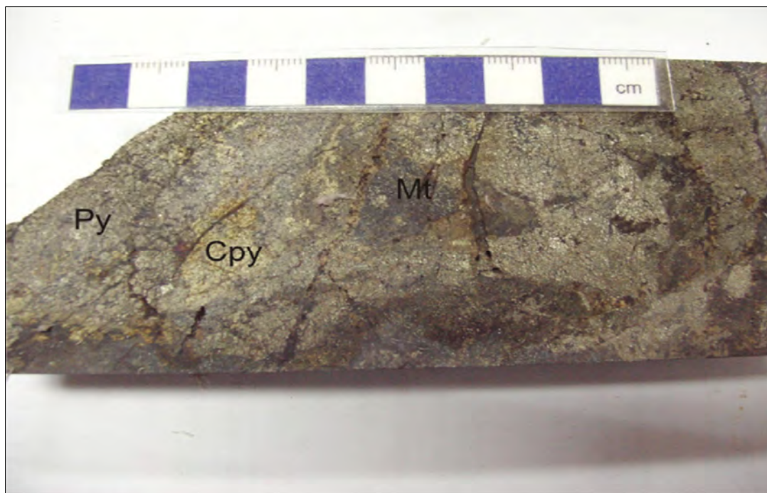
Photograph 32: PUT 2 massive sulphide mineralisation, chalcopryite (~20%) in association with pyrite (~50%) and magnetite (~30%). Assays are unknown. Source: Khositanont, 2007. Visual estimates of mineral abundance should never be considered a proxy or substitute for laboratory analyses where concentrations or grades are the factor of principal economic interest. Visual estimates also potentially provide no information regarding impurities or deleterious physical properties relevant to valuations.
