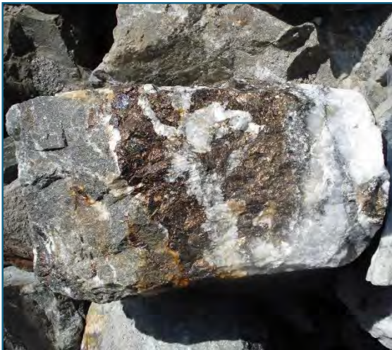
Photograph 14: (Left) 2008 Mesam Gold Mine visit. Mine dump sample of a quartz (~60%) - pyrrhotite (~40%) - chalcopyrite (trace) vein. Source: Author.
