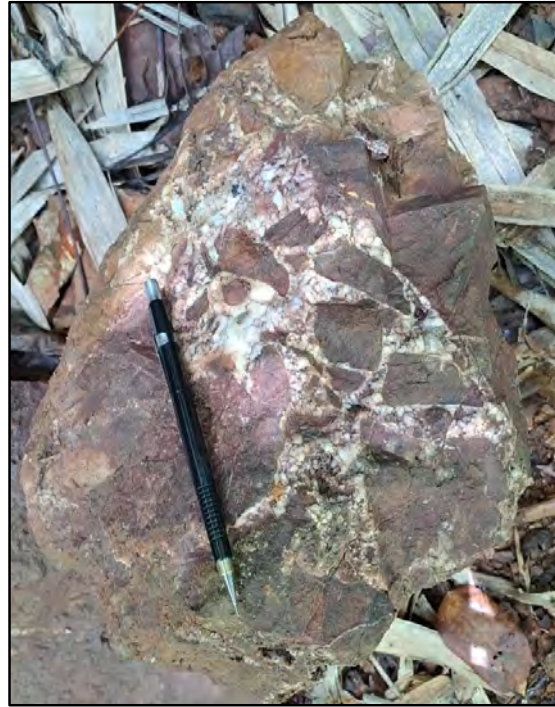
Photograph 2: (Left) Rohav Prospect. Quartz-arsenopyrite vein from Vietnamese artisanal mine. A rock chip sample (ID 103217) taken from this vein at location 685024 m East, 1390919 m North returned assay results of 20.5 g/t gold, 81.7 g/t silver and 0.4% arsenic (refer to Appendix A for all rock chip sample assay results). Source: Author.
