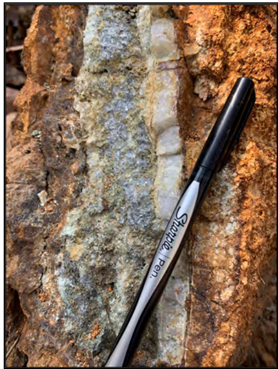
Photograph 21: (Left) Camp Prospect. Brecciated massive arsenopyrite mineralisation hosted in granodiorite from the old mine workings. A rock chip sample (ID O2303032) taken from this mineralisation at location 722747 m East, 1416171 m North returned assay results of 1.2 g/t gold, 24.4 g/t silver and 6.8% arsenic (refer to Appendix B for all rock chip sample assay results). Source: Unity Metals.
