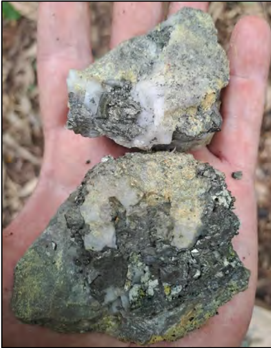
Photograph 2: (Left) Rohav Prospect. Quartz-arsenopyrite vein from Vietnamese artisanal mine. A rock chip sample (ID 103217) taken from this vein at location 685024 m East, 1390919 m North returned assay results of 20.5 g/t gold, 81.7 g/t silver and 0.4% arsenic (refer to Appendix A for all rock chip sample assay results). Source: Author.
