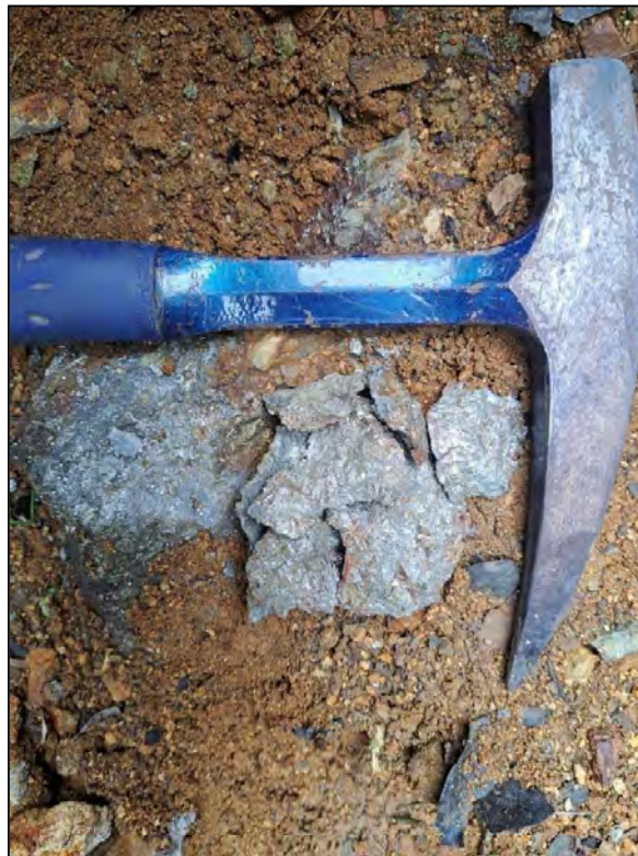
Photograph 26: (Left) Small Creek Prospect. Arsenopyrite-rich mullock adjacent to an old mine working. A rock chip sample (ID O2303062) taken from this mineralisation at location 761997 m East, 1414404 m North returned assay results of 10.7 g/t gold, 32.5 g/t silver, 26.2% arsenic and 232 g/t bismuth (Appendix B for all rock chip sample assay results). Source: Unity Metals.
