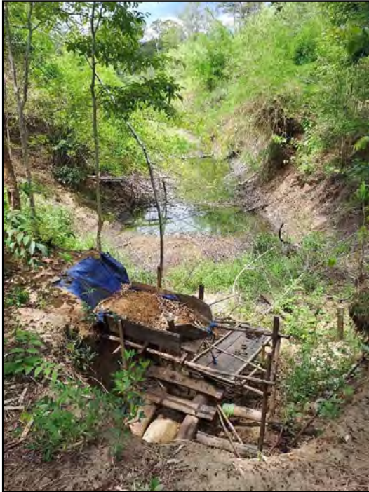
Photograph 23: (Left) Camp Prospect. Artisanal mining gravity table at the eastern end of one of the large 100 m+ long open pits in the northwest portion of the prospect area. Source: Author.
